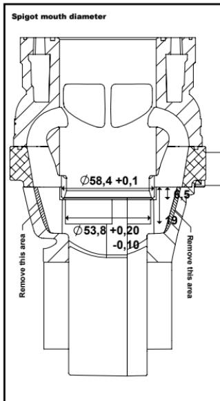
it is necessary to strip the crankcase and revise it in the area around the cylinder base. In order to ensure proper piston clearance, Minarelli engines require the crankcase to be milled in two steps.
