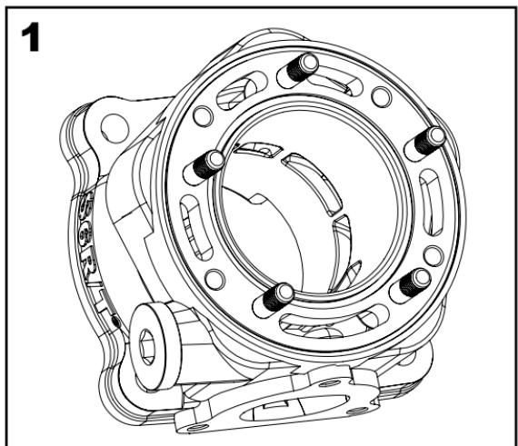
The head cover must be mounted with the water connection opposite the exhaust port and fixed using the four M6 30 mm hexagon socket screws. The supplied copper washer must be placed under the vent plug, which is marked with the inscription *Air* on the head cover.
