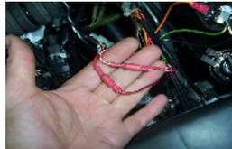
\*CONNECTER LES CABLES ROUGE/BLANC DU DIAGRAMME ET DU STATOR ENSEMBLE. \*CONNECTER LES CABLES NOIR/ROUGE DU DIAGRAMME ET DU STATOR ENSEMBLE.
