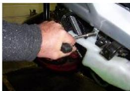
DÉMONTÉ LE VASE D'EXPANSION A L'AIDE D'UNE CLÉ A PIPE DE 10.
