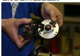
APRÈS AVOIR RETIRÉ LA PLATINE D'ORIGINE, PRÉSENTER LE CABLE DU STATOR MILLÉNIUM PAR LE PASSE FIL DE LA PLATINE ET PRÉSENTER L'ENSEMBLE SUR LE CARTER. LE PASSE FIL DOIT ÊTRE DEVANT LA SORTIE DE CABLE DU CARTER MOTEUR.
