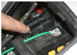
VERIFIER QUE LA BATTERIE EST BIEN EN PLACE AVEC UNE TENSION DE 12 VOLTS.
