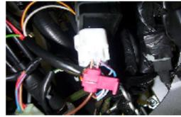
POSITIONNER LE CLIP FOURNI SUR LE CABLE MARRON DU CDI D'ORIGINE SANS LE DÉCONNECTER NI LE COUPER, PLACER LE CABLE MARRON DU DIAGRAMME EN PARALLELE SUR LE CLIP A COTÉ DU CABLE MARRON DU CDI ET FERMER LE CLIP AVEC UNE PINCE POUR QUE LES 2 CABLE SE METTENT EN CONTACT.
