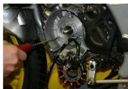
SERRER LES 3 VIS DE FIXATION DE 4 mm FOURNIES A L'AIDE D'UN TOURNEVIS CRUCIFORME.
