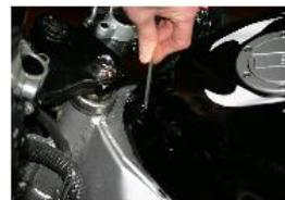
RETIRER LA VIS DE FIXATION AVANT DU RÉSERVOIR AVEC UNE CLÉ ALLEN DE 5.
