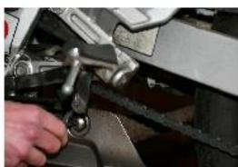
RETIRER LA VIS ARRIÈRE DU CARÉNAGE A L'AIDE D'UNE CLÉ ALLEN DE 4.
