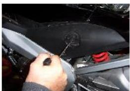
DÉPOSER LE CACHE DE PROTECTION DU ROBINET APRÈS AVOIR RETIRÉ LA MANETTE DU ROBINET AVEC UNE CLÉ ALLEN DE 5.
