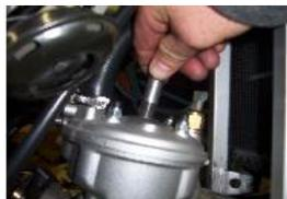
METTRE A LA PLACE DE LA BOUGIE, UN BLOQUE PISTON ET TOURNER A LA MAIN LE ROTOR D'ALLUMAGE POUR METTRE LE PISTON EN CONTACT AVEC
