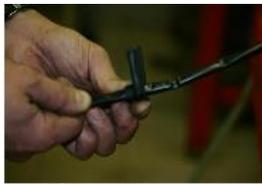
APRÈS AVOIR RÉCUPÉRÉ L'OBTURATEUR SUR LA GAINÉ DU STATOR D'ORIGINE, LE POSITIONNER DANS LE BON SENS SUR LA GAINÉ DU STATOR MILLÉNIUM.
