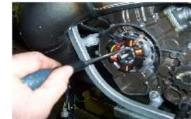
RETIRER LES 3 VIS DE FIXATION DU STATOR AVEC UN TOURNEVIS CRUCIFORME.
