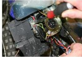
POSITIONNER LA BOBINE HAUTE TENSION A SON EMBLACEMENT D'ORIGINE EN FIXANT A LA MASSE LE CABLE NOIR DU DIAGRAMME ET VERT/JAUNE DU STATOR.
