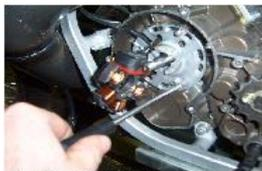
ATTENTION!! LES 3 VIS DE LA PLATINE SONT PARTICULIÈREMENT DIFFICILES A DESSERRER, POUR CE FAIRE, PRÉSENTER UNE CLÉ ALLEN DE 3 ET TAPOTER AVEC UN MARTEAU SUR LA CLÉ AVANT D'ESSAYER DE LA DESSERRER.
