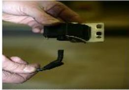
VISSER LE CABLE SUR LA BOBINE HAUTE TENSION ET RABATTRE LA PROTECTION SUR LA BOBINE ET CONNECTER LE CABLE ORANGE DU DIAGRAMME SUR LA COSSE D'ALIMENTATION DE LA BOBINE.
