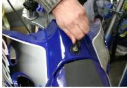
OUVRIER LE CACHE RÉSERVOIR AVEC LA CLÉ DE CONTACT.
