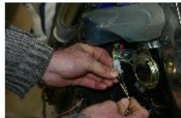
SUR LE MEME CONNECTEUR, BRANCHER LE CABLE NOIR/BLANC DU DIAGRAMME AVEC LE VERT/NOIR DU CONNECTEUR. FIXER LE DIAGRAMME AU DESSUS DE LA BOBINE AVEC UN COLLIER PLASTIQUE ET RASSEMBLER TOUS LES CABLES AVEC 3 COLLIERS PLASTIQUE.
