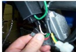
RETIRER LES CABLE DE LA BOBINE HAUTE TENSION ET DECONNECTER LE CONNECTEUR 2 VOIES BLANC RELIANT LE STATOR D'ORIGINE AU FAISCEAU
