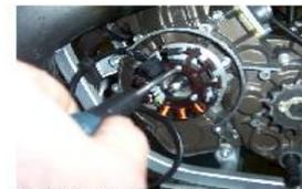
PRÉSENTER LE STATOR MILLÉNIUM SUR SA PLATINE EN PASSANT LA GAINÉ PAR LE TROU DU CARTER ET LE SERRER AVEC LES 3 VIS DE 4 mm FOURNIES AVEC UN TOURNEVIS CRUCIFORME.
