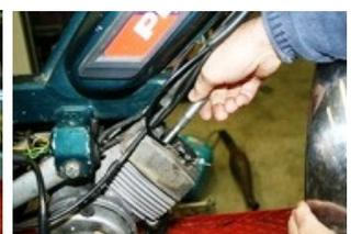
Unscrew the stick and place back the spark plug and the connector cap.
