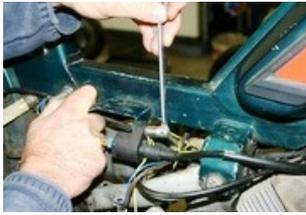
Remove the screw of the high voltage coil and the mass wire.
