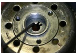
There is two position on the MVT rotor, A=analogic and D=digital. With this ignition use the A position.
