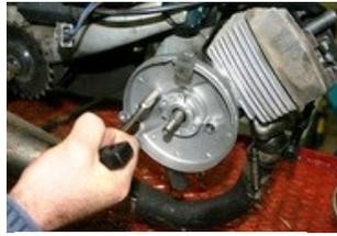
Remove the screws of the original ignition support.
