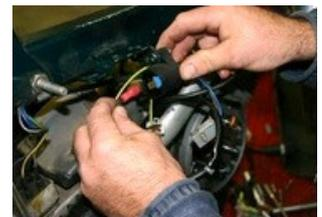
Connect the black wire from the Premium stator on the blue pod of the high voltage coil.
