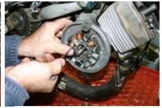
Fit the stator on the engine with the two screws 5x30 delivered with the ignition.
