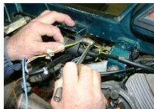
Fit all the mass wires together on the metal body of the MVT high voltage coil with an 8mm key.
