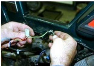
Joint the mass wire of the MVT stator with the originals mass wires to the metal body of the MVT high voltage coil.
