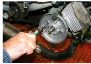
Fit the support with the two screws 6x20 milled heads and control if the support is correctly on the engine without any screws of casing does not obstruct.
