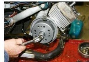
Screwed the rotor with the original screw on the crankshaft.
