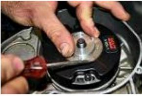
1\_Turn the crankshaft in the rotation side of the engine to block the piston on the stick
