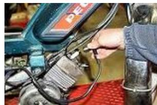
Connect the blue wire from the DIGITAL DIRECT stator with the white wire of the
