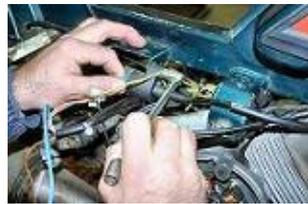
Fit all the mass wires together on the metal body of the MVT high voltage coil with an
