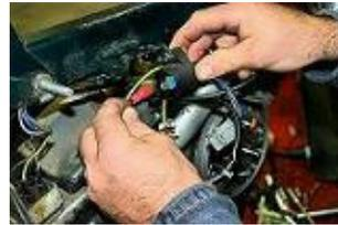
Connect the black wire from the DIGITAL DIRECT stator on the pod of the high voltage coil.
