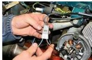
Connect the Yellow wire with the brown wire of the stator.
