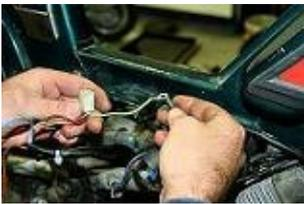
Joint the mass wire of the MVT stator with the originals mass wires to the metal body of the MVT high voltage coil.
