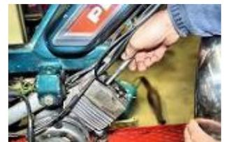
Unscrew the stick and place back the spark plug and the connector cap.
