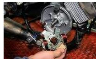
Remove the stator
