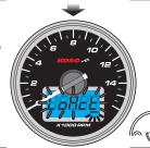
Press the **Adjust button** to choose the input signal you want to set. Now the input signal setting is flashing!
