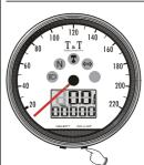
●In trip B screen, press the Adjust button once to switch from trip B to clock screen
