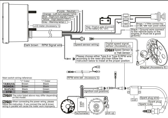
When connecting the power wiring, please follow the instruction. If you connect the red & brown wiring in parallel will cause the meter work improperly.
