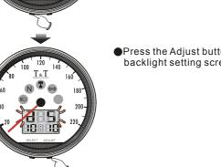
●Press the Adjust button to choose the backlight setting screen.
