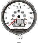
Press the Select button once to enter the external odometer setting screen.
