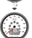
●Press the Adjust button to choose the external odometer setting screen.
