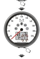
●Enter the number of ignition signals per crankshaft revolution ( "P" value). This may vary according to the vehicle manufacturer/model and type of engine:
