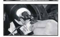
4. Disconnect the wiring from the speedometer, tachometer, ambient temp.meter, volt meter, fuel meter, and oil pressure meter.
