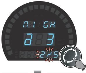
●**EX** : The backlight brightness (night) setting is changed from 3/5 (60%) to 2/5 (40%).
