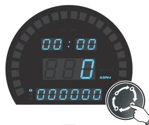
●In the total mileage screen, press the button once to switch to Trip A screen.
