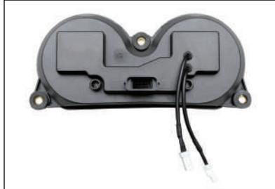
9. Re-use the bushings and nuts to install the KOSO speed/tachometer
