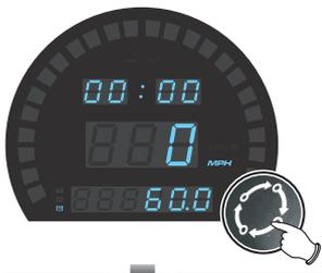
• In the Trip B screen, press the button once to switch to the mileage maintenance screen.
