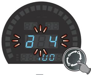
●In the tire circumference screen, hold the **button for 3 seconds** to enter into the settings screen.
