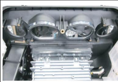
5. Ensure the Speed and Tach bezels remain in the fairing.
