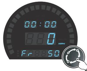
• In the tire pressure screen, press the button once to switch to the MAX. record screen.
