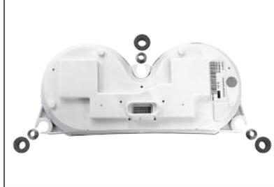
8. Remove the bushings and nuts from the original Speedometer and Tachometer.
