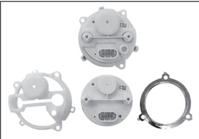
6. The Fuel and Volt bezels and mounting cups will be reused. There are 3 tabs on the bezels that need to be carefully pushed back through the mounting cup to separate the bezel from the mounting cup and to release the factory gauge.
