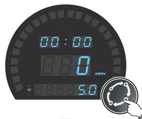
●Trip A screen, press the button once to switch to Trip B screen.
