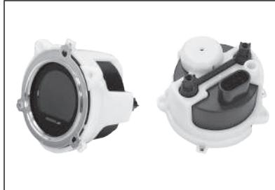
7. The new OIL TEMP gauge will use the existing white Volt mounting cup and the new Fuel Level gauge will use the existing black Fuel mounting cup. Place the new VOLT and OIL TEMP gauge in the appropriate housings and secure the bezel in place by lining up the tabs.
