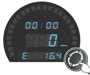
• In the average fuel consumption screen, press the button once to switch to the tire pressure screen.
