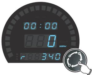
• In the remaining mileage screen, press the button once to switch to the average fuel consumption screen.
